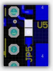
In case if for supply used USB connector or pogo pins, JP5 must be close in this position
