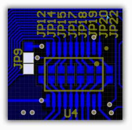
2.2 I/O lines used for signals with 3.3V logic levels.
